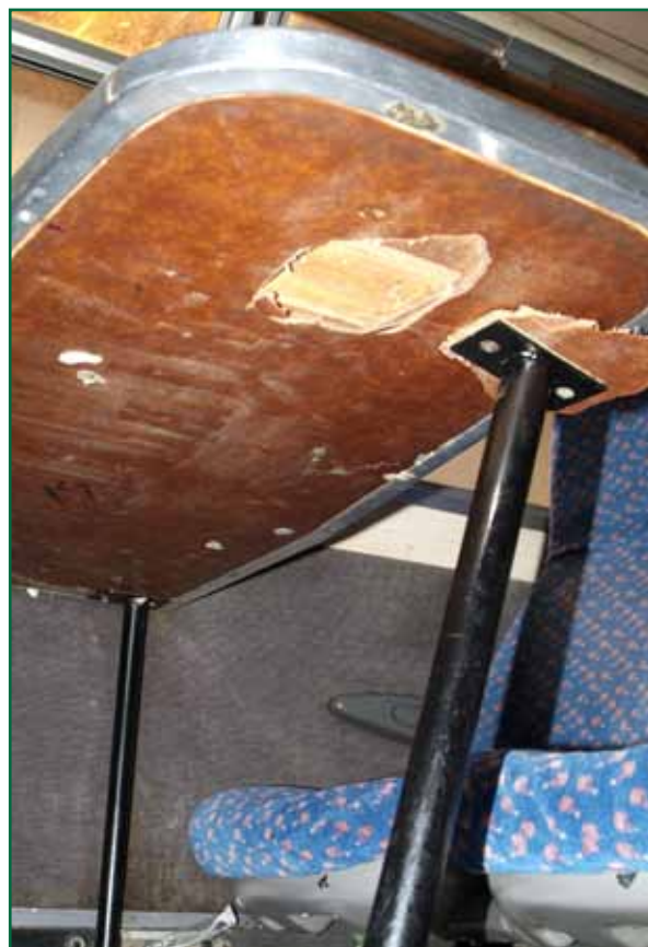
Figure 14: Typical example of table deflection
